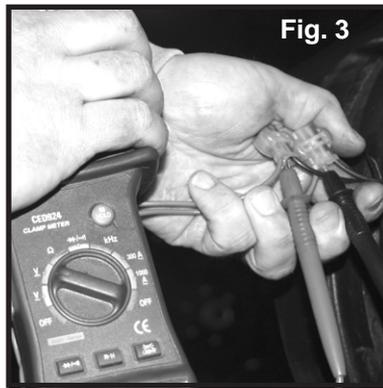
Taking a Voltage reading is usually done with probes inserted into the wire connector (See Fig. 3).
